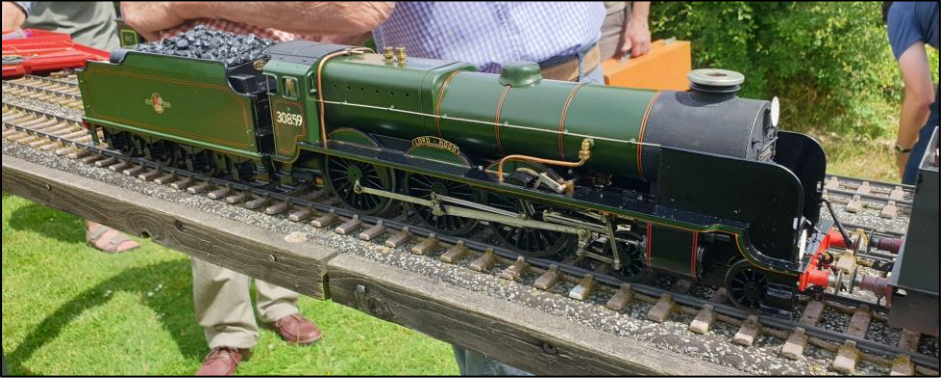
SR Lord Hood, the soft cushion for the steam raising blower still in the chimney.
